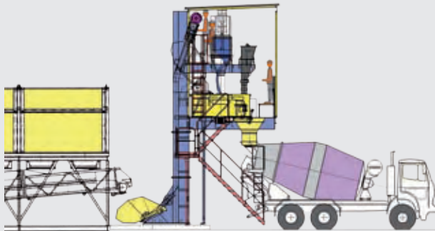
Design as in-line silo (bin), 4 to 10 compartments possible, with storage volume of 70 to 300 m³.
