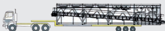
Vehicle 3: In-line silo (bin) with belt weigher.
