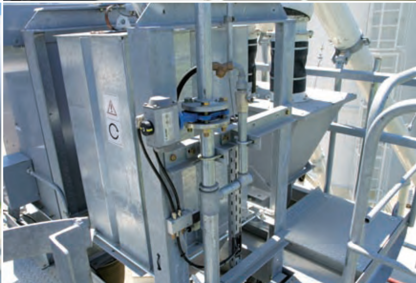
The large-scale weighing platform, with cement and water weighers, has good maintenance access.
