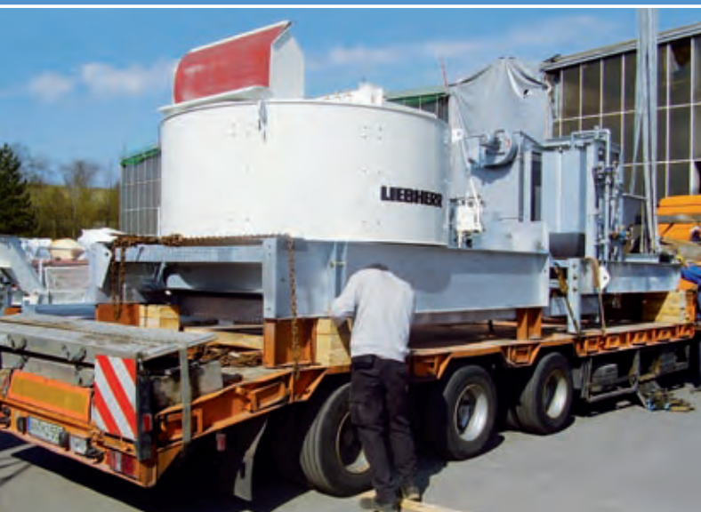
Vehicle 1: Mixing and weighing platform with walls of the in-line silo (bin).
