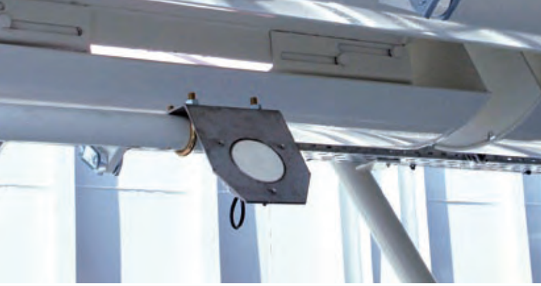
Litronic-FMS II moisture measuring system for assessing sand moisture content.
