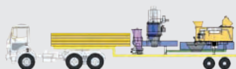
Vehicle 1: Mixing and weighing platform with walls of the in-line silo (bin).
