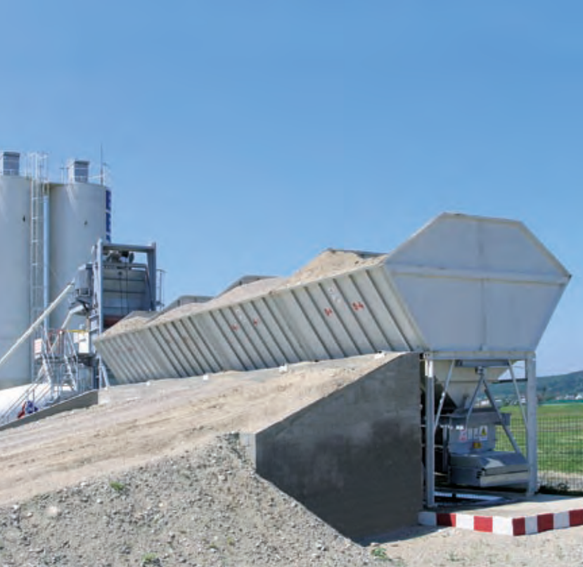
Design as in-line silo (bin), 4 to 10 compartments possible, with storage volume of 70 to 300 m³.
