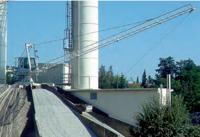
Design as star-pattern aggregate bays, 4 to 6 compartments possible, total storage volume approx. 950 m³
